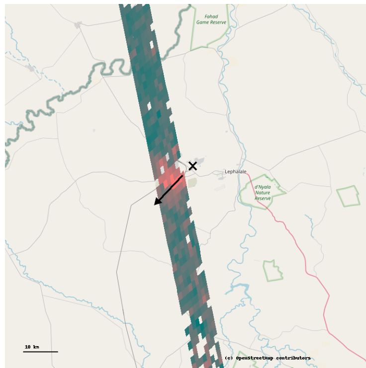
Figure 1 – plume identified on a portion of an OCO-2 orbit over South Africa centred on sounding 2014110711502571 (v10 retrievals, plotted over an OpenStreetmap background). The cross marks the Matimba coal power plant and the arrow shows the wind direction.
