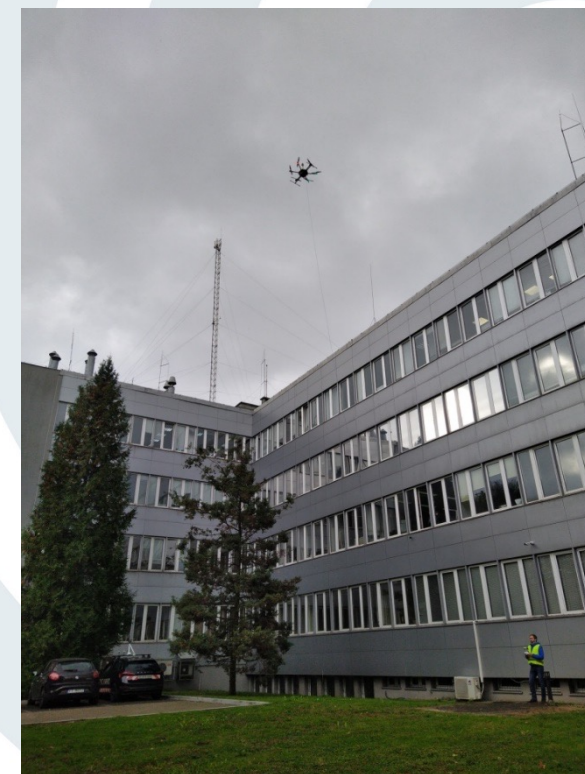
A 200m long tube connected the drone with the analyzer.
